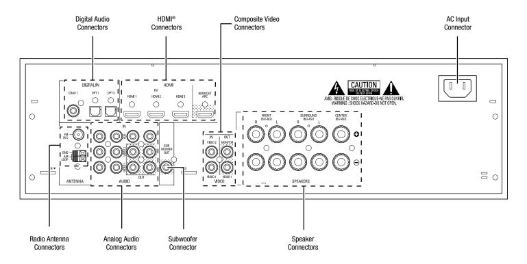
**Radio Antenna connectors:** Connect the included AM and FM antennas to their respective terminals for radio reception. See *Connect the Radio Antennas*, on page 13, for more information.
