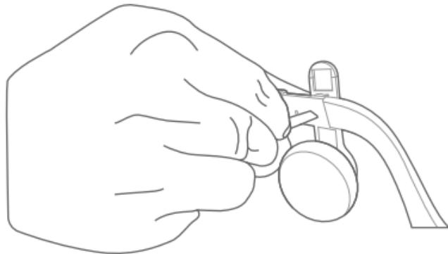
4. Turn the audio tool clockwise (to the right) to tighten the screw until it is secure.
