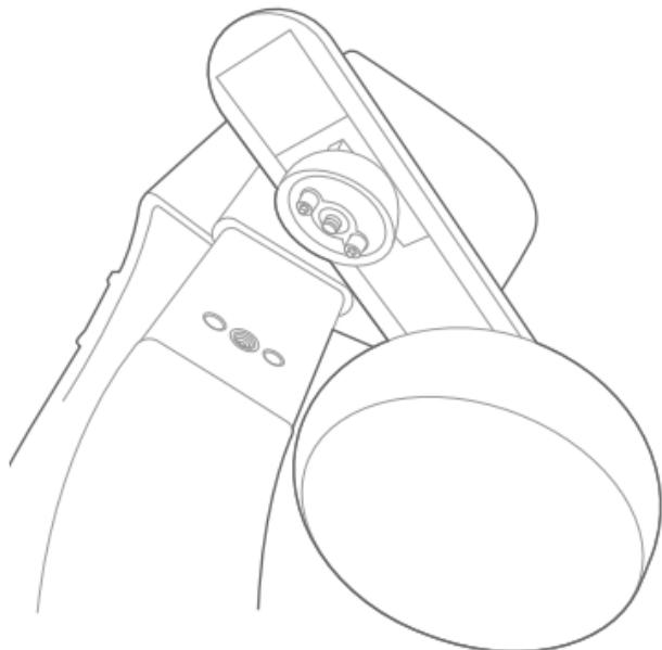
2. Place the head of the audio arm into the screw and hold it in place.
