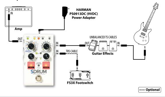
**NOTE:** When only the AMP OUT jack is used, the drum signal will be processed to make the drums sound better when played through a guitar amp. See 'Output Jack Operation' on page 10 for more information. If using guitar effects and/or a looper in this type of application, they should be placed before the SDRUM so they do not affect the drum signal. Note that the effects may need to be bypassed to use BeatScratch.
