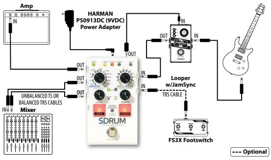
**NOTE:** The looper should be placed before the SDRUM in most cases, such as when using only the AMP OUT jack. if using the AMP and MIXER OUT jacks, the looper can also be placed between the SDRUM and amp if desired. See 'Using JamSync' on page 31 for information on using the SDRUM in a JamSync setup.
