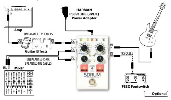
**NOTE:** When connected to both the MIXER and AMP OUT jacks, the guitar signal will be fed to the AMP OUT jack and the drum signal will be fed to the MIXER OUT jacks. See 'Output Jack Operation' on page 10 for more information. If using guitar effects, they can be placed before the SDRUM or between the SDRUM and amp in this type of application. Note that if the effects are placed before the SDRUM, they may need to be bypassed to use BeatScratch.
