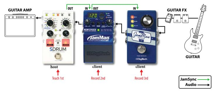
**NOTE:** When cascading audio through multiple JamMan loopers in series and using JamSync (as shown in the diagram above), the SDRUM (the host) should be last in the chain in most cases. You will then want to teach the SDRUM first, then record to the second to last device, etc., working backwards through the signal chain. Performing these actions will ensure you record only what you intend to during each pass.
