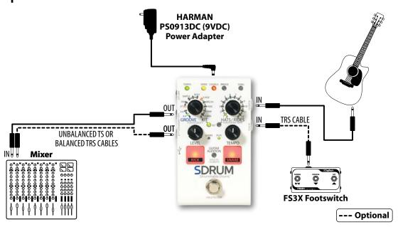
**NOTE:** When only the MIXER OUT jacks are used, the mono guitar signal and stereo drum signal are fed to the MIXER OUT jacks. This setup works well for applications where an acoustic guitar with a pickup or a bass guitar are connected to a live PA system. See *'Output Jack Operation'* on page 10 for more information.
