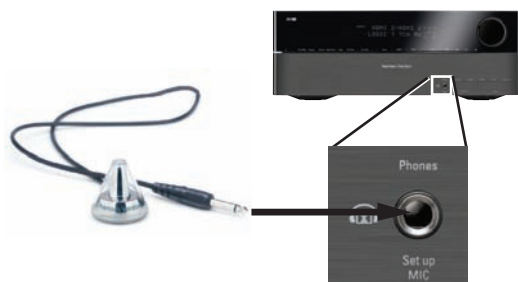
Figure 51 – Plug EzSet/EQ microphone into receiver.
