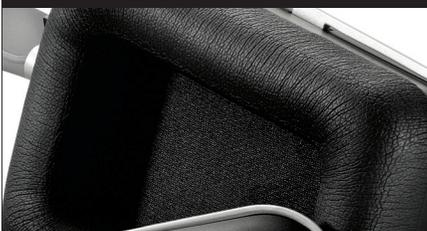
Premium foam in the ear pads contributes to the BT headphones' excellent passive noise reduction and extended bass response. The slow-retention foam helps maintain an acoustic seal around the ear, which keeps outside noises out and also keeps the listener's music from disturbing others.
