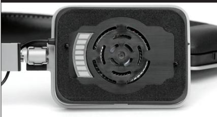
High-performance 1-5/8-inch (40-millimeter) drivers produce an excellent frequency response (16Hz – 20kHz), wide dynamic range and high sound-pressure levels. As a result, BT headphones deliver accurate sound and extended bass response.
