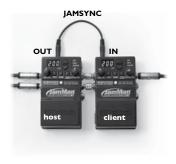
To use JamSync, connect the host JamMan Solo XT's JAMSYNC OUT jack to the JAMSYNC IN jack of the first client device. Daisy chain any remaining JamSync client in the same manner.
