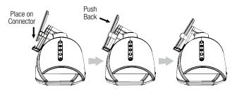
To dock an iPad device, press the lock button on the back of the dock and extend the base of the dock, then follow steps 1 and 2 above.
